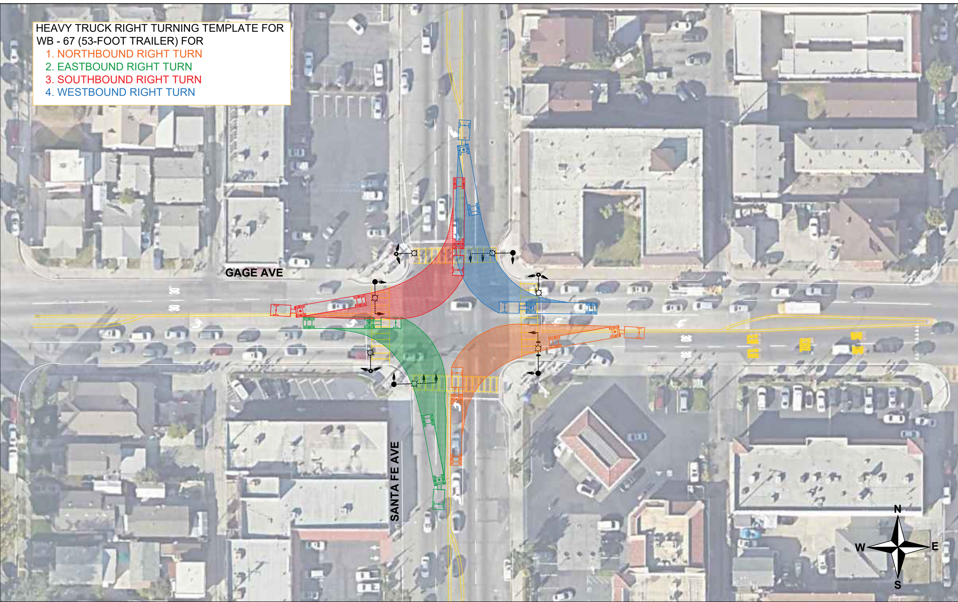
Intersection 6: Gage Ave and Santa Fe Ave - Truck Right Turning Template
