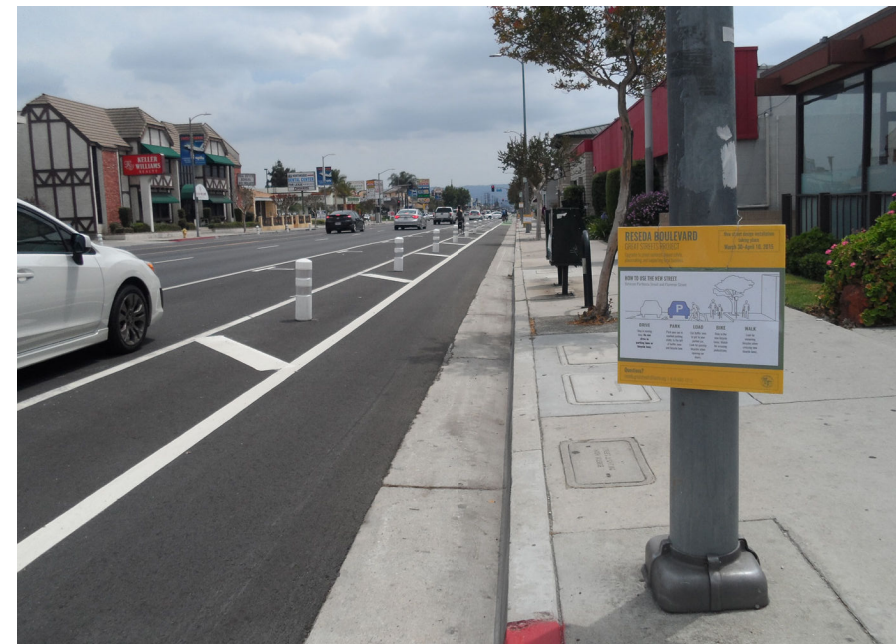
FIGURE 40: EXAMPLE OF BUFFER WITH BOLLARDS
