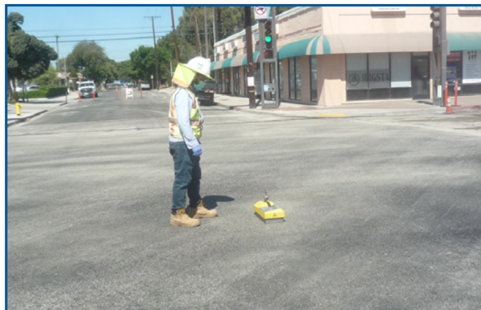
Ninyo & Moore Technician does compaction test on asphalt.
