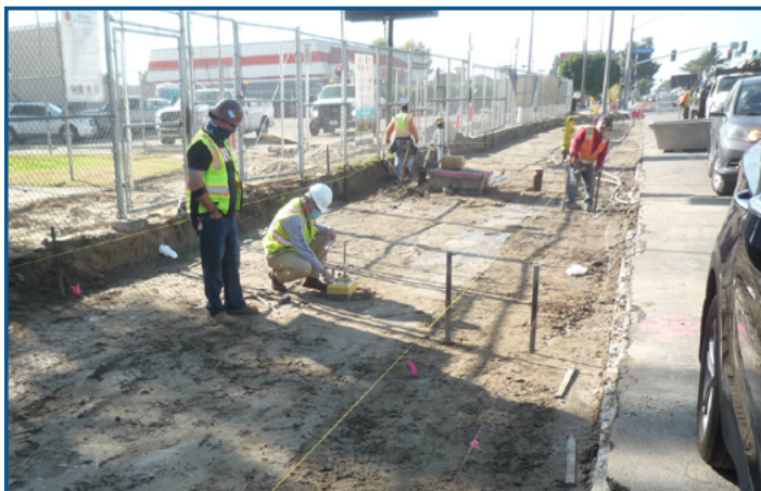
Ninyo & Moore Technician does compaction test on base.
