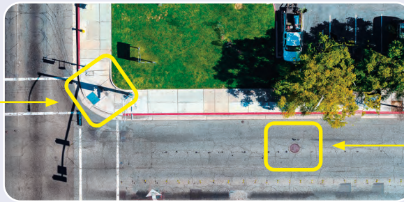
MANHOLE ASPHALT UPHEAVAL
